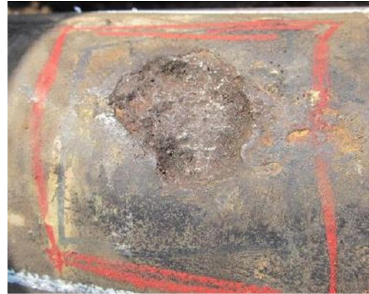
Corroded void
